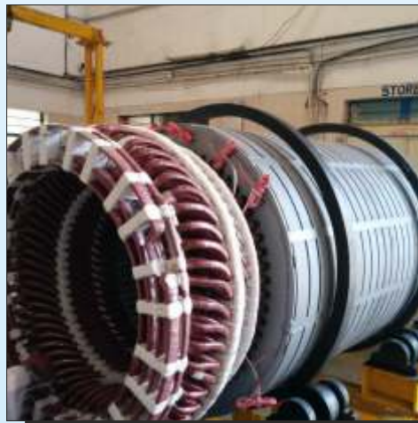
6MVA,6.6KV, Stator Winding
