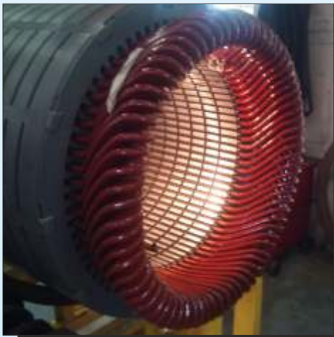
6MVA,6.6KV, Stator Post Winding
