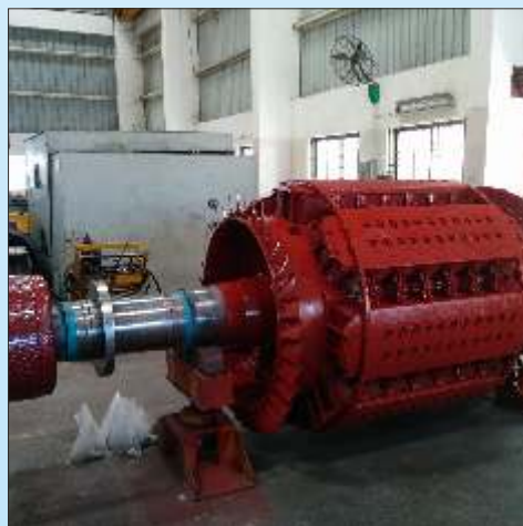
7.5MVA,6.6KV, Alternator Strip On Edge Rotor Winding
