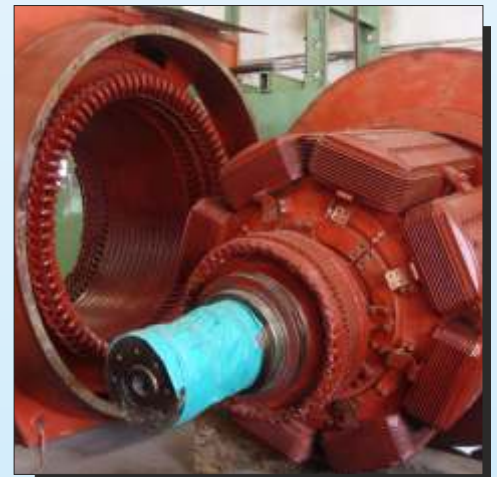
8MVA,11KV, Stator & Rotor
