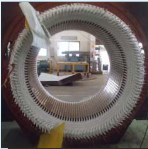
6MVA,6.6KV, Stator Post Rewinding
