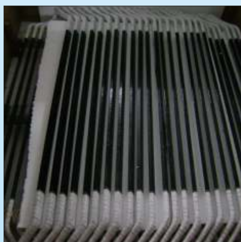
11KV, Roebel Bars
