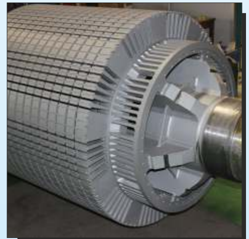
6MVA, Rotor Core Assembly
