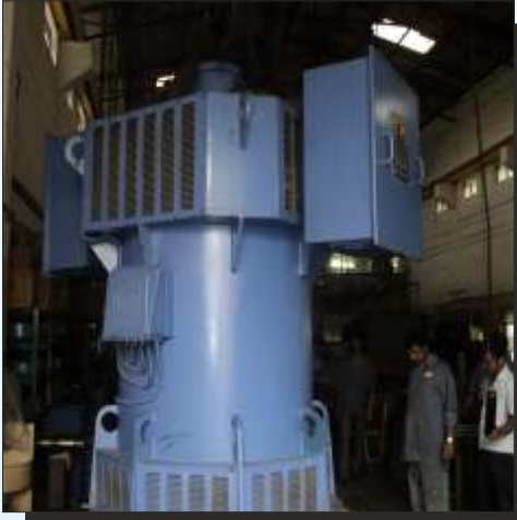
1.75 MVA, 8 Pole, Alternator Run Test
