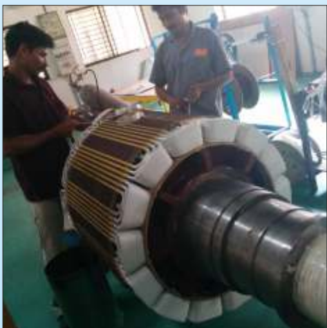
6MVA,6.6KV, Salient Pole Rotor Rewinding
