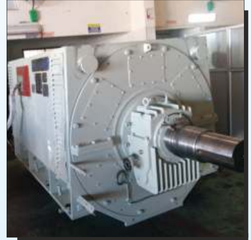
10.5MW, 6.6KV, Motor
