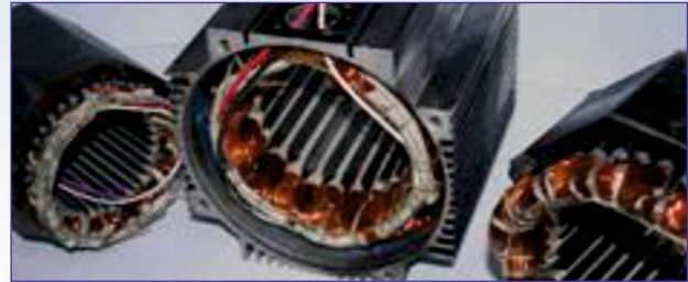
Rewinding of Servo Motors
