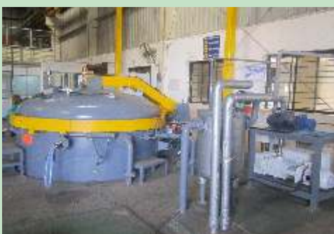
2-VPI PLANTS 1.5 Mtr Dia x 2.0 Mtr . Height 2.5 Mtr Dia x 3.0 Mtr. Height
