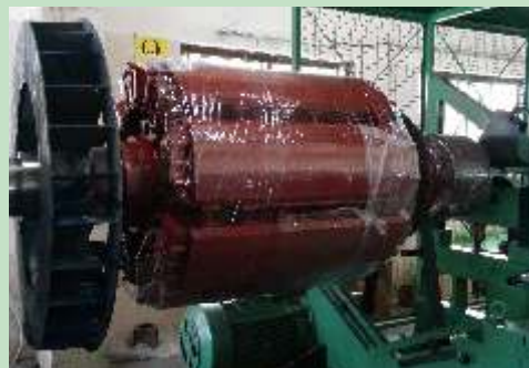
18 TON DYNAMIC BALANCING MACHINE 9 Mtr LENGTH
